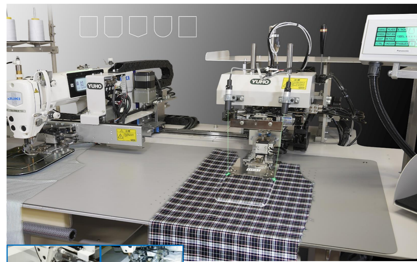
Right: Custom Gauge for L/R Symmetric Pockets (Optional) Left: Custom Gauge for Double-Stitch (Optional)
